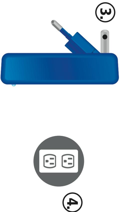
**4.** Plug USB CHARGER into Wall Outlet. Blue LED Light will illuminate to indicate power.
